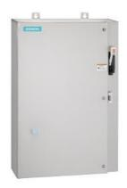
Non-reversing motor starter Size 1 Three phase full voltage Solid-state overload relay OLRelay amp range 0.75-3.4A 240VAC 50HZ / 277VAC 60HZ coil Combination type 30Amp non-fusible disconnect Encl NEMA type 4X 316 S-steel Water/dust tight non-corrosive Extra-wide enclosure
