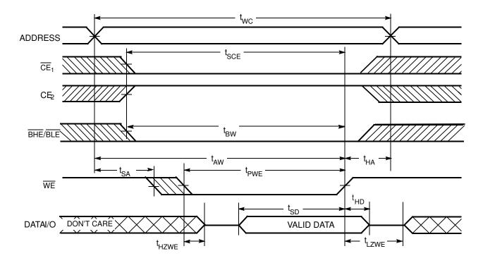
Write Cycle No. 4 (BHE/BLE Controlled, OE LOW)<sup>[18, 19]</sup>
