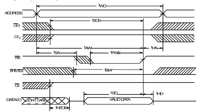
Write Cycle 2 ( $\overline{CE}_1$  or  $CE_2$  Controlled)<sup>[12, 13, 17, 18, 19]</sup>
