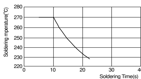
[Allowable Flow Soldering Temperature and Time]
