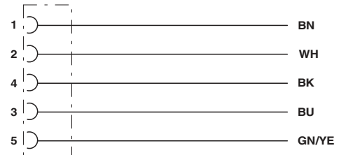
Contact assignment of the M12 sockets
