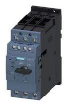
Circuit breaker size S2 for motor protection, CLASS 10 A-release 12...17 A N-release 260 A screw terminal Standard switching capacity with transverse auxiliary switches 1 NO+1 NC
