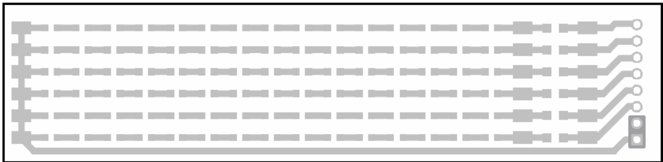
Figure 2—LED Board Top Layer
