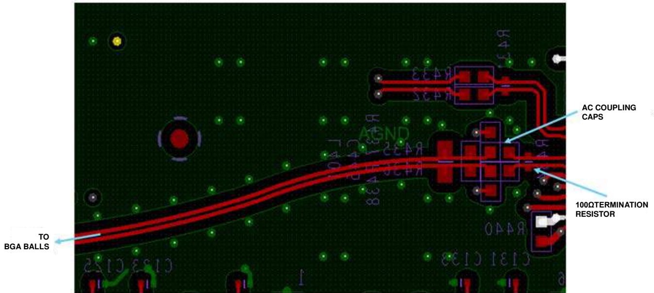
Figure 173. REF_CLK_IN \pm Routing Recommendation
