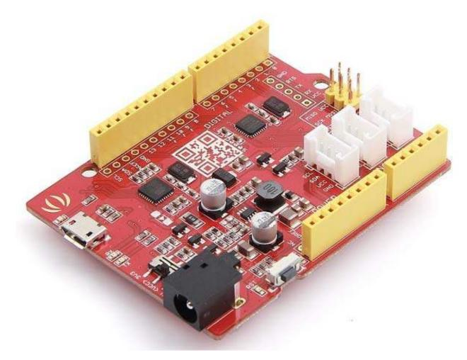
Seeeduino v4.2 is an Open Source, Arduino-compatible ATmega328 MCU development board. We think Seeeduino v4.2 is one of the best Arduino derivatives/compatibles available. Seeeduino v4.2 is feature rich, much more stable, easy-to-use and even good looking.
