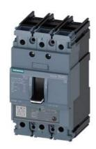
circuit breaker 3VA5 UL frame 125 breaking capacity class S 25kA @ 480 V 3-pole, line protection TM230, FTAM, In=60A overload protection Ir=60A fixed short-circuit protection Ii=5...10 x In UL489 SB (naval), 50 deg. cel. nut keeper kit on both sides
