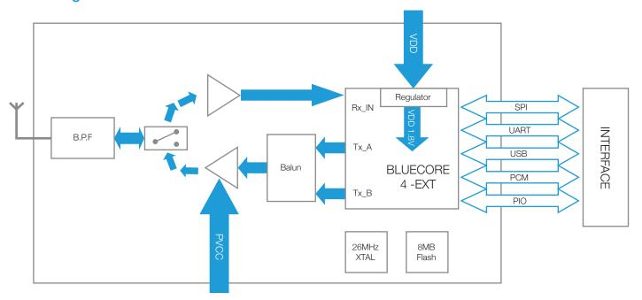
Note: USB and PCM interface are not handled by LM firmware at present
