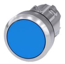
Pushbutton, 22 mm, round, metal, shiny, blue, pushbutton, flat, latching, Push-to-release mechanism, with laser labeling, lower case
