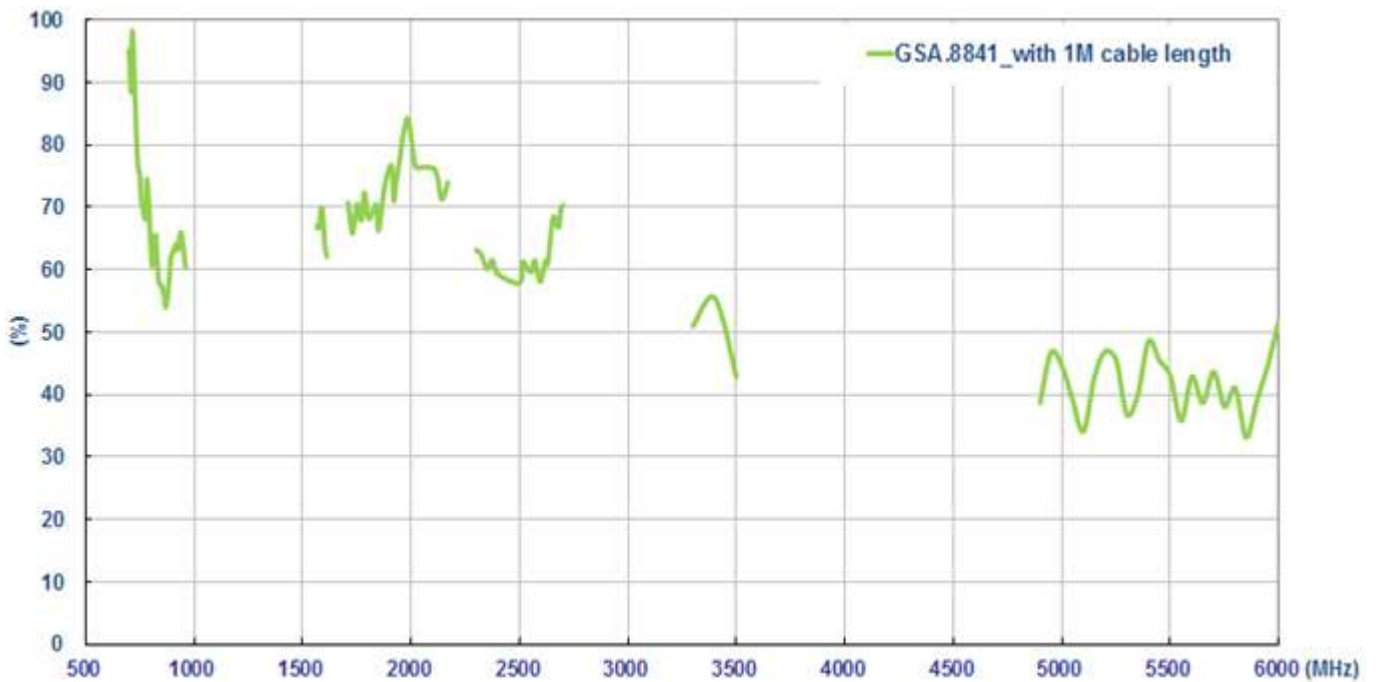
Figure7. Efficiency of GSA.8841 with 1 meter cable length on the glass base
