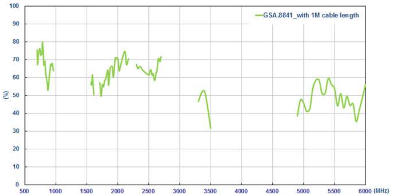
Figure5. Efficiency of GSA.8841 with 1 meter cable length in free space
