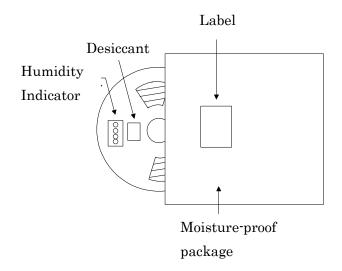
Reel will be packed in moisture-proof package together with desiccant and humidity indicator. After packing, the package will be heat-sealed.
