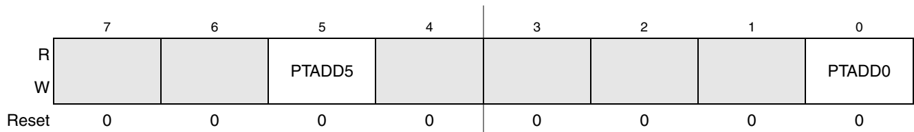
Figure 6-3. Data Direction for Port A Register (PTADD)
