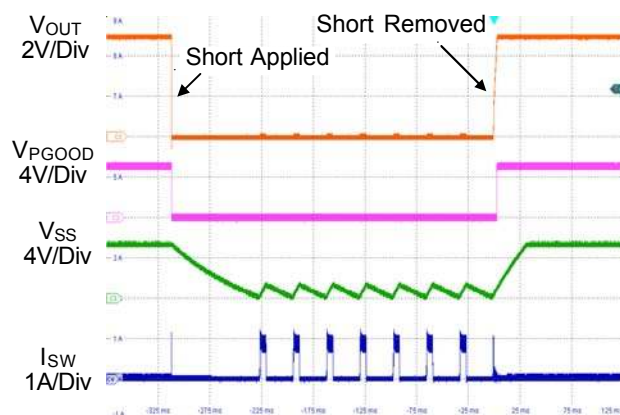
Figure 3. Short Circuit Protection and Recovery
