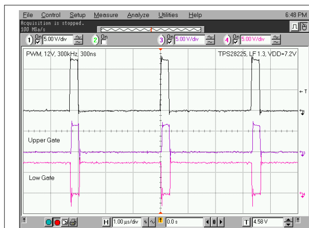
Figure 7-4. 12-V PWM Pulse at V_{DD} = 7.2\text{ V}
