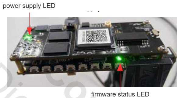
figure 3-4 position and definition of LEDs
