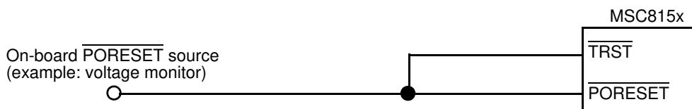
Figure 35. Reset Connection in Functional Application
