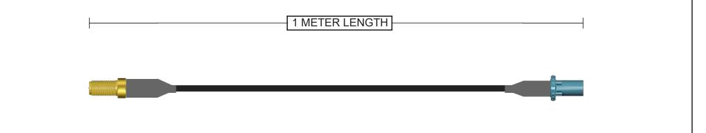
Connector A 132116RP SMA Jack Straight Brass Gold + Heatshrink 50 Ohm RG-58 Continuity/Hi-Pot Connector B 2FA1-NZSP-C04Y1 FAKRA Plug Straight Zinc Nickel + Heatshrink
