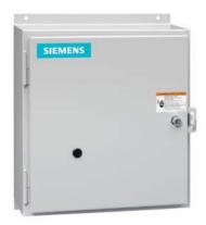
Mechanically held lighting contactor, Contactor amp rating 100Amp 0NC  $\_2NO$  poles, 24VAC 60HZ coil, Non-combination type, Enclosure NEMA type 12, Dust/drip proof for indoors
