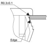
Process the above-mentioned R on the mounting hole side of panel, or be sure that the Play R is on the operation side of panel when using. Be sure that the Edge is on the reverse side of panel when processing.
