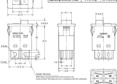
**Note:** Unless otherwise specified, a tolerance of  $\pm 0.3$  mm applies to all dimensions.
