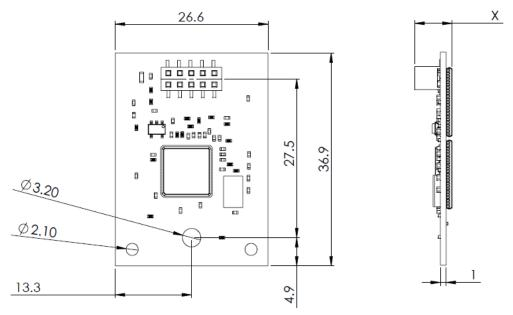
All dimensions in mm. Tolerance on all dimensions  $\pm\,0.5\text{mm}.$
