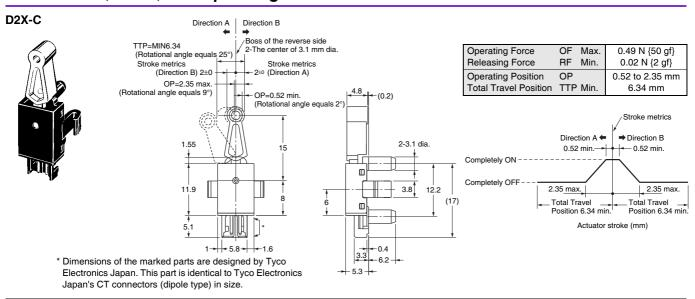
Note 1. Unless otherwise specified, a tolerance of  $\pm 0.4$  mm applies to all dimensions.
