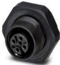
Sensor/actuator flush-type connector, socket, 5-pos., M12, A-coded, rear/screw mounting with Pg9 thread, with solder cups, plastic version
