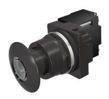
30mm BlackMax, Epoxy Coated Corrosion Resistant Complete Metal Unit Illuminated Push-Pull Operator Full Voltage, 120V AC/DC Incandescent Lamp Mushroom Head Cap Small 1 3/4" (44.5 mm) Metal, Black with Clear Lens 3 Position Momentary UL Listed, CSA Certified NEMA 1,3,3R,4,4X,12,13 & Automotive Standards
