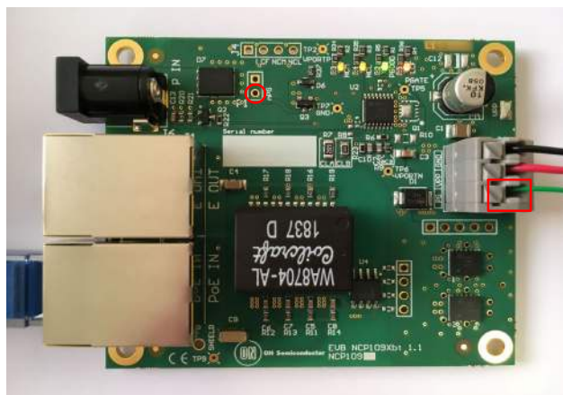
Figure 1. Operational NCP1096GEVB Showing Basic Interconnections
