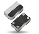
The ITF High Directivity Wide Band LGA Coupler is based on thinfilm multilayer technology. The technology provides a miniature part with excellent high frequency performance and rugged construction for reliable automatic assembly. The Wide Band High Directivity Coupler displays a stable coupling factor over a wide frequency band.
