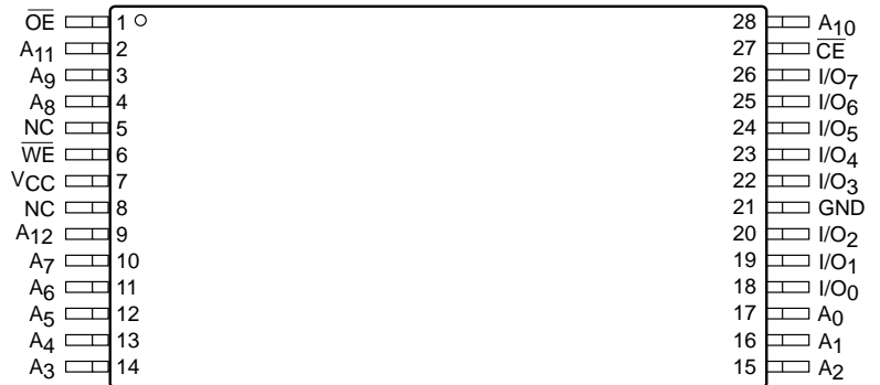
TSOP Top View (8mm x 13.4mm) (H13)
