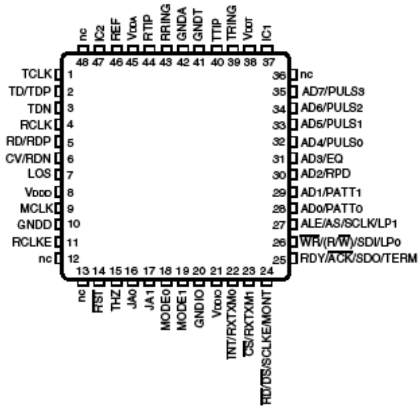
Figure-3 IDT82V2081 NLG Package Pin Assignment
