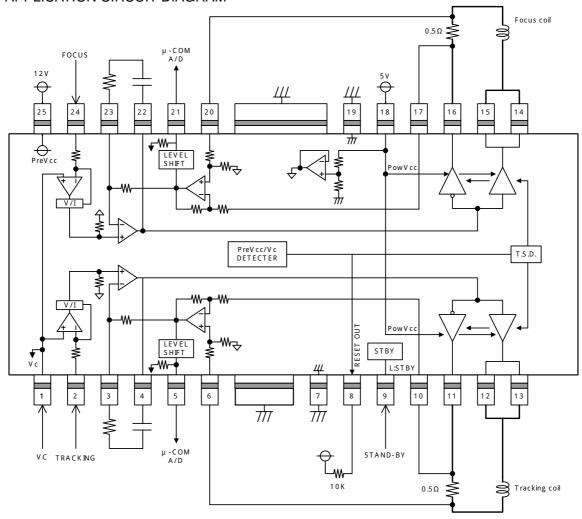
T.S.D: (Thermal shutdown) Resistance unit:  $[\Omega]$
