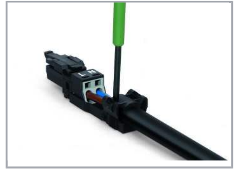
Push down strain relief clamp with 2.5 mm screwdriver alternately on both sides.
