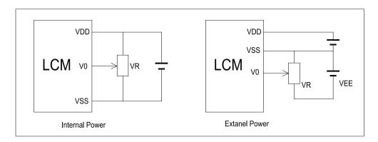
V<sub>DD~</sub>V₀: LCD Driving voltage
