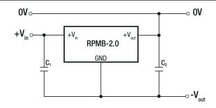
$\mathbf{C_1}$  and  $\mathbf{C_2}$  may be added to reduced ripple and should be fitted close to the converter pins.
