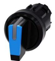
Selector switch, illuminable, 22 mm, round, plastic, blue, selector switch, short, 3 switch positions I>O<II, momentary contact on the left, latching on the right, actuating angle  $2x45^{\circ}$ , 10:30h/12h/13:30h, with laser labeling, upper case
