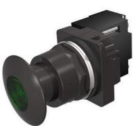
30mm BlackMax, Epoxy Coated Corrosion Resistant Complete Metal Unit Illuminated Push-Pull Operator Full Voltage, 24V AC/DC Incandescent Lamp Mushroom Head Cap Small 1 3/4" (44.5 mm) Metal, Black with Green Lens 3 Position Pull-Momentary/Push-Maintained UL Listed, CSA Certified NEMA 1,3,3R,4,4X,12,13 & Automotive Standards
