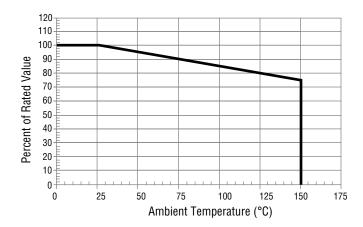
This graph shows the typical device surge current derating versus ambient temperature when subjected to the 8/20 µs current waveform per the IEC 61000-4-5 specification. This device is not intended for continuous operation at temperatures above 125 °C.
