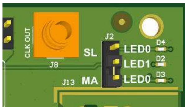
Figure 2-6. DP83TC812 configured as Master
