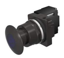
30mm BlackMax, Epoxy Coated Corrosion Resistant Complete Metal Unit Illuminated Push-Pull Operator Full Voltage, 6V AC/DC Incandescent Lamp Mushroom Head Cap Small 1 3/4" (44.5 mm) Metal, Black with Blue Lens 3 Position Pull-Momentary/Push-Maintained UL Listed, CSA Certified NEMA 1,3,3R,4,4X,12,13 & Automotive Standards
