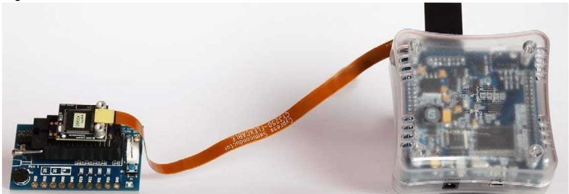
Figure 3-10. Flex Pod Connected to ICE-Cube Pod
