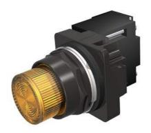
30mm BlackMax, Epoxy Coated Corrosion Resistant Complete Metal Unit Illuminated Indicator Light Full Voltage type, 120V AC/DC Incandescent Lamp, BA9s Plastic Lens, Amber UL Listed, CSA Certified NEMA 1,3,3R,4,4X,12,13 & Automotive Standards
