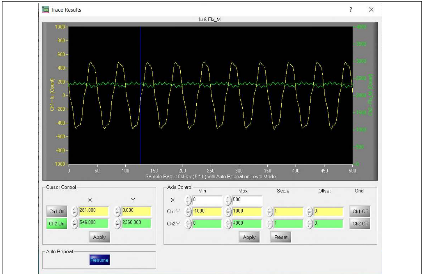
Figure 10 Trace waveform for Iu & Flx-M at 50% speed
