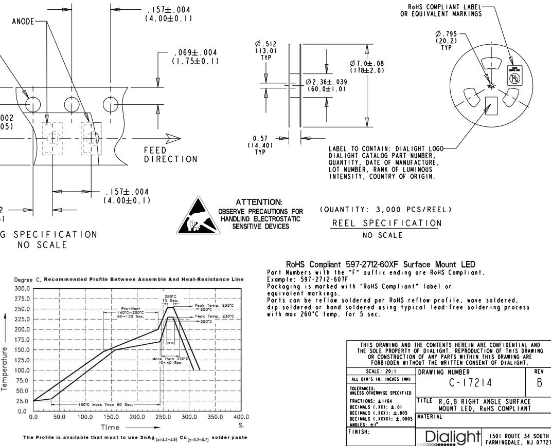
The Profile is available that must to use SnAg  $_{(x=3,3\sim3,8)}$  Cu  $_{(y=0.2\sim0.7)}$  solder paste
