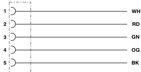
Contact assignment of 7/8" plugs/sockets, cable type 410
