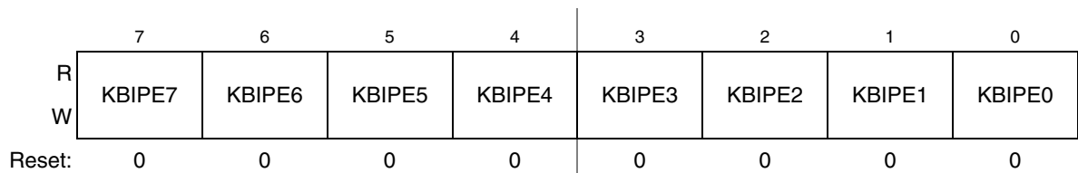
Figure 9-4. KBI Pin Enable Register
