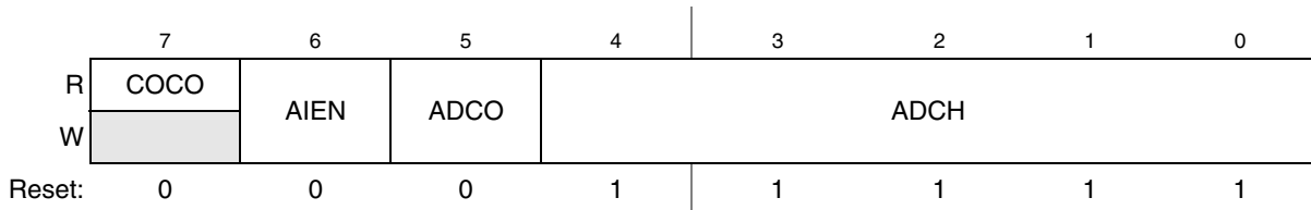
Figure 10-3. Status and Control Register (ADCSC1)
