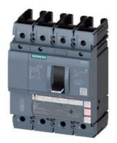
circuit breaker 3VA5 UL frame 250 breaking capacity class H 65kA @ 480V 4-pole, line protection TM210, FTFM, In=100A overload protection Ir=100A fixed short-circuit protection Ii=10 x In N conductor unprotected without connection
