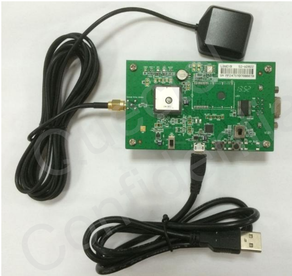
Figure 9: EVB and Accessory Equipment
