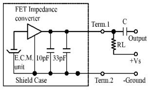
RL =  $2.2 \text{ k}\Omega$ C =  $1 \mu\text{F}$
