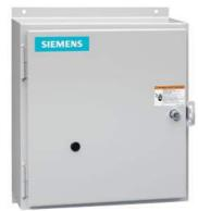
Mechanically held lighting contactor, Contactor amp rating 20Amp 0NC  $\_$  6NO poles, 208-240V 50/60HZ coil, Non-combination type, Enclosure NEMA type 12, Dust/drip proof for indoors
