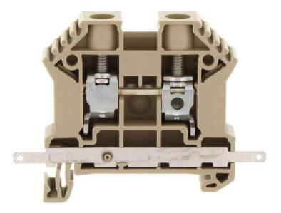
Feed-through terminal, Screw connection, Mounting type: Mounting rail TS 35/7.5, Rated cross-section: 16 mm<sup>2</sup>, Width: 10 mm, Colour: Orange
