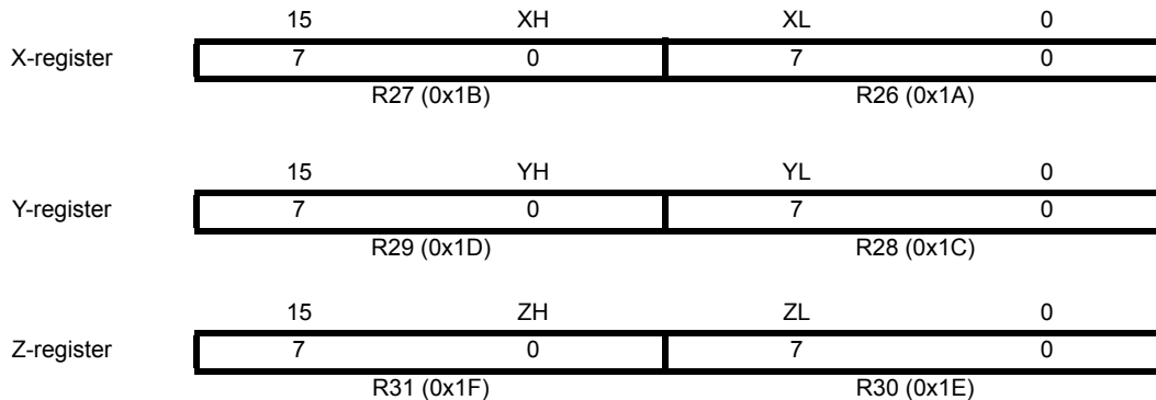
Figure 4-3. The X-, Y-, and Z-registers
